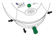
Figure 4. Inserting a Pad-Pak
